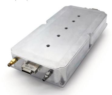
is multi-paction free TNC female. Transmit test data appears on page two of this data sheet at room temperature. This SSPA operates from -40C to +85C baseplate temperature. The configuration shown is hermetically sealed. This SSPA can also be vented.
