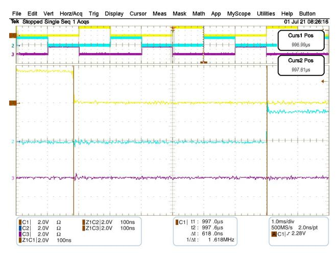
Figure 4: Minimum Dead-Band Delay between two GPIO pins
