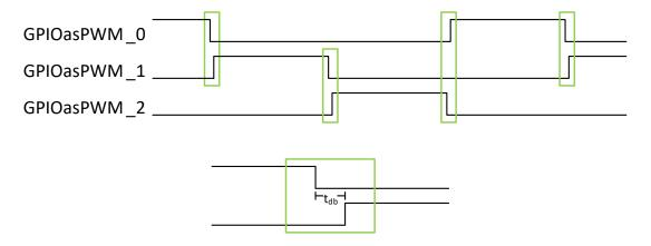
Figure 3: Dead Band time (t<sub>db</sub>) between alternating PWM signals
