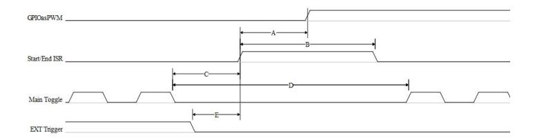
Figure 6: Delays Within various Interrupt Service Routines
