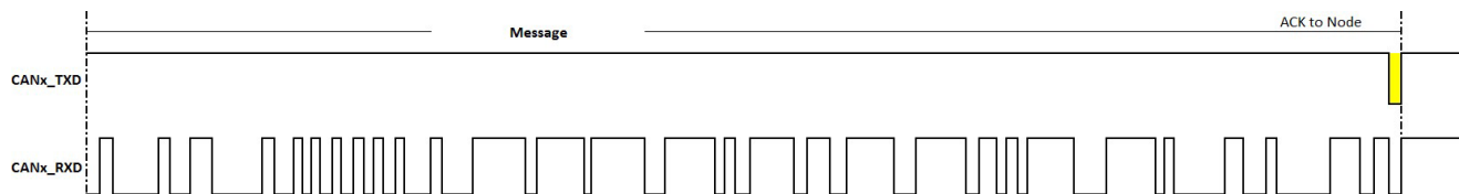
Figure 13: PeliCAN receiving message from a Node
