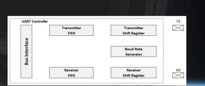
The message starts with first, the Start bit by driving the tx line low for one clock cycle. Second, data is transmitted in the next 8 clock cycles bit by bit with optionally sending the parity bit in the 9 clock cycle. Finally, the stop bit by pulling the tx line high to end the transmission
