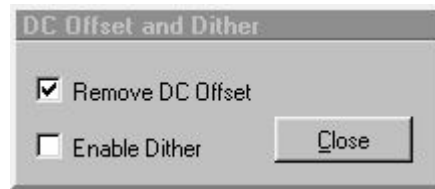
Fig. 9 DC offset and dither control
