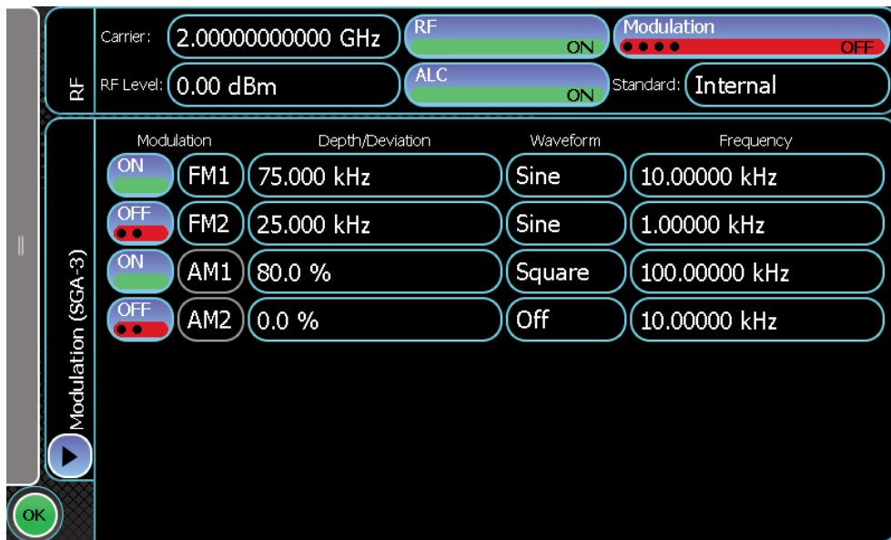
Typical multiple modulation set-up
