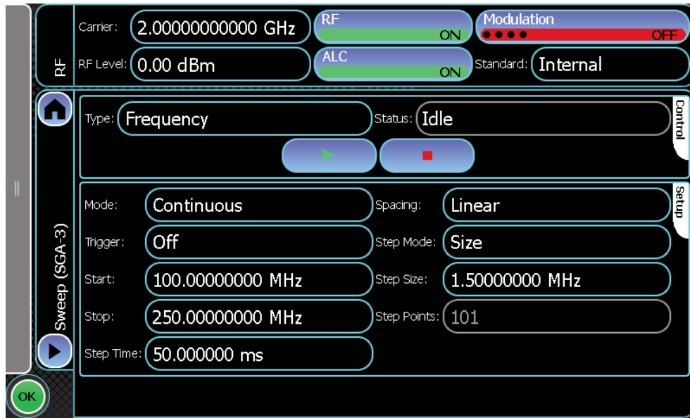
Typical frequency sweep set-up
